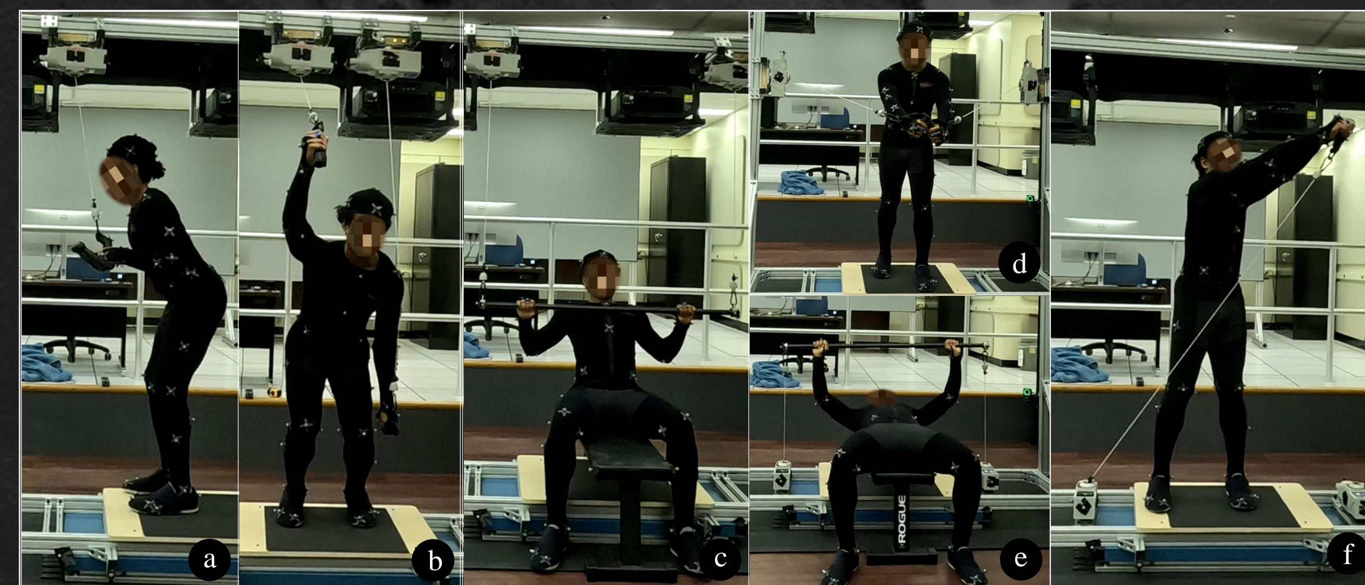
Figure 1. NGED modalities. a) Tricep extension exercise with a single top-mounted Beyond Power Voltra I system b) Alternating-hand ski exercise with dual top-mounted Voltra I systems c) Lat pulldown with dual top-mounted Voltra I systems d) Fly exercise with dual shoulder-level Voltra I systems e) Bench press exercise with dual ground-mounted Voltra I systems f) Reverse-chop exercise with a single ground-mounted Voltra I system
