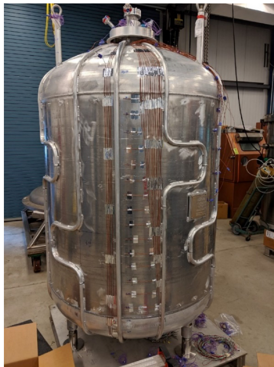
Figure 12.—CryoFILL tank resting on its feet on pallet.
