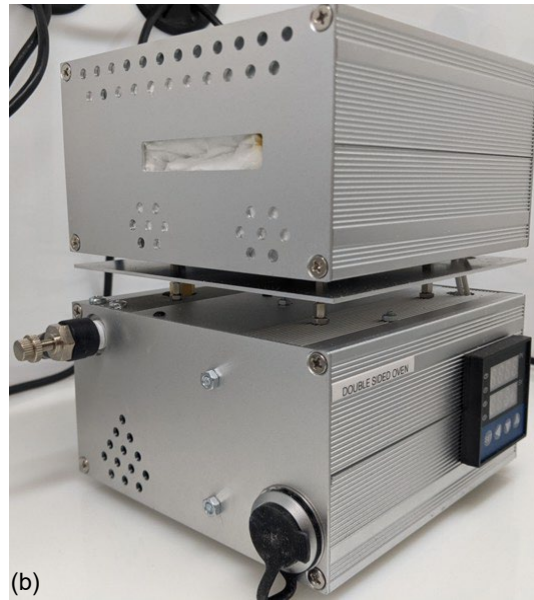
Figure 8.—Back of Mark II oven. (a) Single-sided version. (b) Double-sided version.
