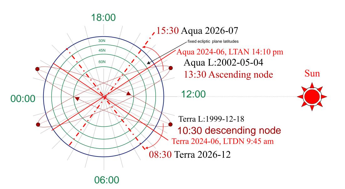
Diagram showing Sun-synchronous orbits from a top view of the local time zones for reference and descending /ascending nodes of 10:30 am and 13:30 pm, and their evolution.
