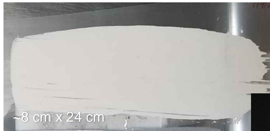
Tape-Casted LPSC Films (~25 \mu\text{m} thickness)
