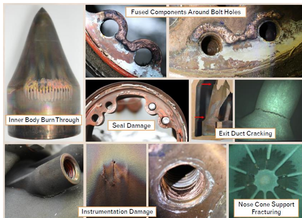
Fig 8. Damage of hardware from single wave operation.
