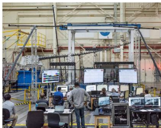
Passive Aeroelastic Tailored Wing heavily instrumented with FOSS technology for shape sensing during load testing.
