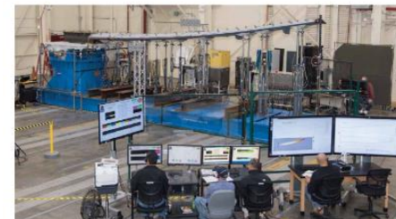
Application of FOSS for wing loads calibration and shape sensing
