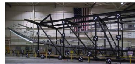
Global Observer Wing instrumented with FOSS for shape sensing
