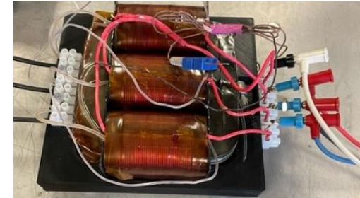
3.3 kVA single-phase design (3x for 10 kW)
