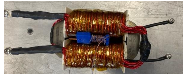
3.3 kVA single-phase design (3x for 10 kW)
