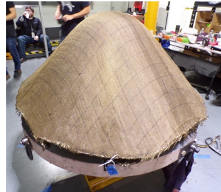
Formed and trimmed sphere-cone preform
