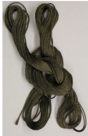
Twisted and stretch-broken yarn
