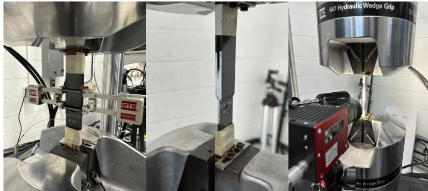
Figure 74 – Double Lap Shear Test Setup
