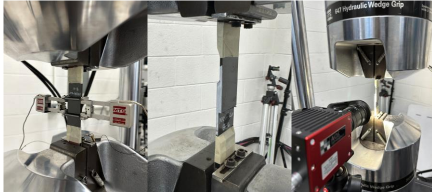
Figure 63 – Single Lap Shear Test Setup
