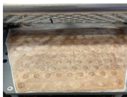
Using Piezo electric to remove water from fecal matter, for laundry, and water recycling. ( Bigalow ICES-2024-287)
