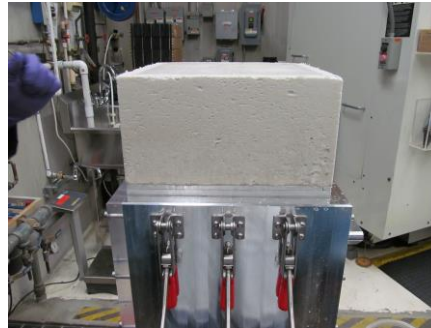
12-inch casting tower
