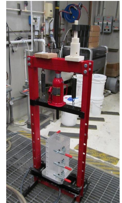
4-inch casting tower
