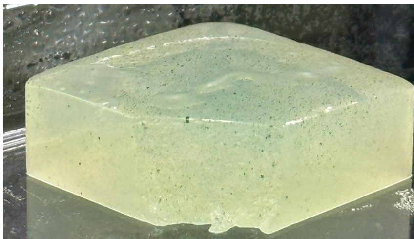
Figure 20. Algal hydrogel bricks. Through qualitative assessment, we found that the alga Chlamydomonas reinhardtii can grow within hydrogel bricks. This finding is important for our ultimate goal of producing living materials composed of symbiotic interactions between algae and fungi.
