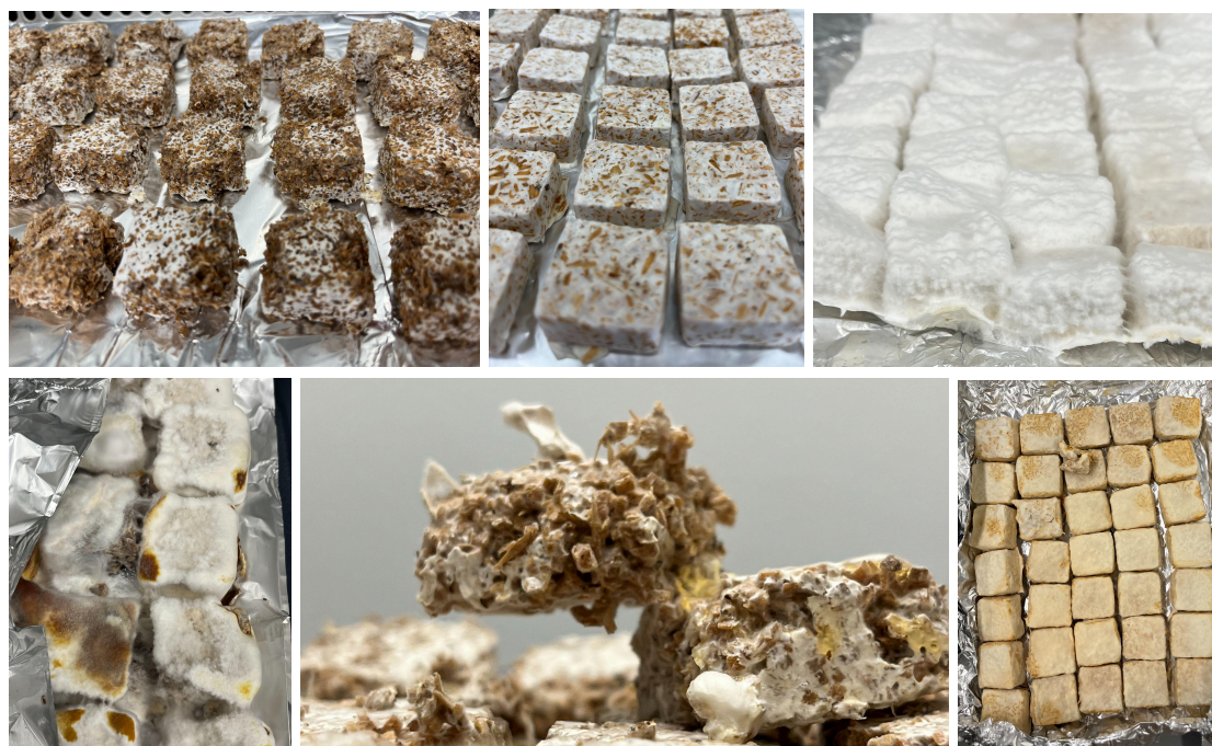
Figure 15. Lignocellulosic biomass-based mycelium materials. We developed a system to explore various species and substrate combinations for material production. We used a commercially available mycelium material as a reference material for developing our own in-house strain and substrate.
