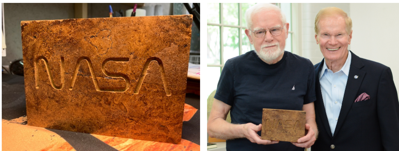
Fig. 1. Left: Bio-Brick made of Myco-Architecture Materials (Courtesy Chris Maurer): This brick is a composite of wood and fungal mycelium. Fungi break down biochemicals like cellulose converting them into their own chitin-rich biomass. By growing mycelium on plant fodder they fuse at a cellular level allowing us to utilize the best characteristics of their respective Kingdoms - Plantae and Fungi. We are currently developing methods to grow these multi-kingdom composites off-planet to save transport cost, reduce energy demands, and utilize bio-performative aspects such as radiosynthesis, that may one day convert space travel's biggest liability, ionizing radiation, into a resource for material production. Bio-Brick dimension is 17 x 12.5 x 5.5 cm. Right: J. Head and NASA Administrator Bill Nelson examine one of our Bio-Bricks at Brown University. Photo by RI Senator Jack Reed.
