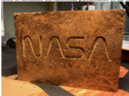
Fig. 1. Left: Bio-Brick made of Myco-Architecture Materials (Courtesy Chris Maurer): This brick is a composite of wood and fungal mycelium. Fungi break down biochemicals like cellulose converting them into their own chitin-rich biomass. By growing mycelium on plant fodder they fuse at a cellular level allowing us to utilize the best characteristics of their respective Kingdoms - Plantae and Fungi. We are currently developing methods to grow these multi-kingdom composites off-planet to save transport cost, reduce energy demands, and utilize bio-performative aspects such as radiosynthesis, that may one day convert space travel's biggest liability, ionizing radiation, into a resource for material production. Bio-Brick dimension is 17 x 12.5 x 5.5 cm. Right: J. Head and NASA Administrator Bill Nelson examine one of our Bio-Bricks at Brown University. Photo by RI Senator Jack Reed.
