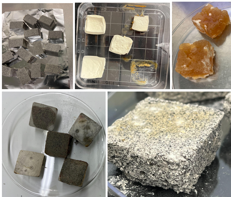
Figure 16. Agar hydrogel-based simulated lunar regolith materials and fungal composites.
