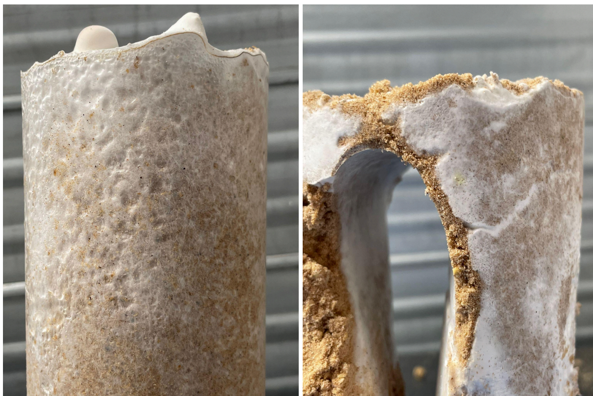
Figure 25. Cylindrical mycelium-sand composites, comprising 85% w/w sand to biomass (mycelium pre-grown on beechwood). Left: A basic cylindrical column, Right: A cylindrical column with an arch, exploring the feasibility of introducing openings and diverse shapes into the components.
