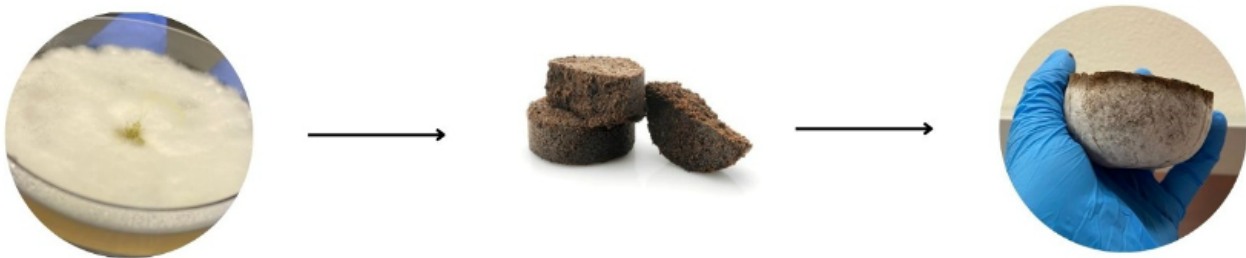
Figure 59. From Aspergillus oryzae agar inoculum to coffee ground wasted, used by Massa to produce a mycelium cup
