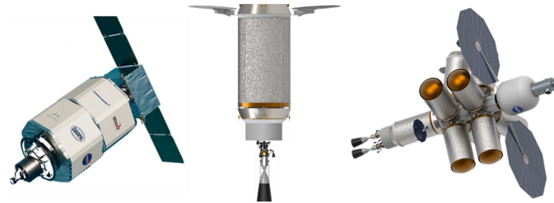
Figure 2: Generational NTP spacecraft – (left) DRACO technology demonstration spacecraft, (center) notional Gen 1/Gen 2 NTP stage, (right) notional multi-NTP engine crewed Mars vehicle with multiple propellant tanks. (images not to scale)
