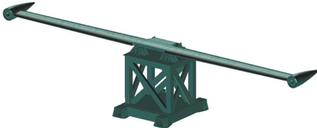
Config A - Mod III wing with cruise motor nacelles, mounted on WLTF
