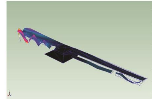
84.43 Hz Anti-sym aileron bending and AW1T
