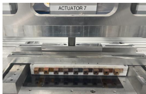
Figure 14 – DCB Manufacturing Setup
