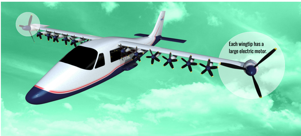
Figure 5. Concept image of Mod IV, the X-57 Maxwell Airplane with the cruise propellers and the high-lift propellers operating [Source: NASA / Advanced Concepts Lab].
