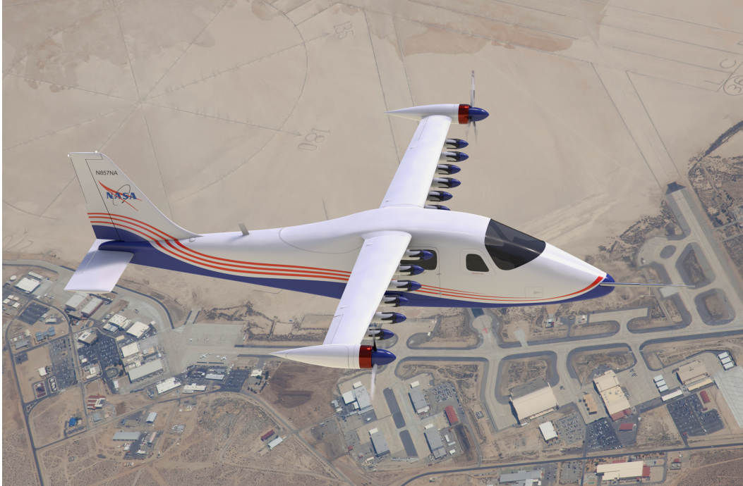
Figure 4. Concept image of Mod III, the X-57 Maxwell Airplane with the cruise propellers operating and the high-lift propellers stowed [Source: NASA / Advanced Concepts Lab].
