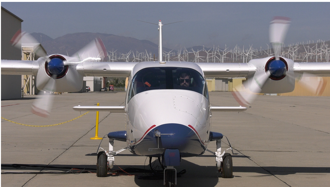
Figure 3. Mod II, the Tecnam P2006T Airplane with electric cruise motors [Source: NASA AFRC TV / Steve Parcel].
