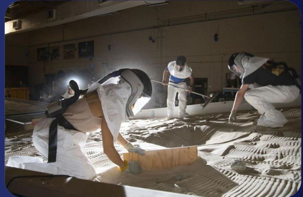
Simulant preparation for VIPER testing at NASA GRC (Credit: NASA).
