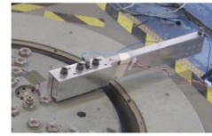
Configuration 1 – Beam without the mass f \approx 300 Hz, M = 6.5 Lb., M_{CL} \approx 4 Lb.
