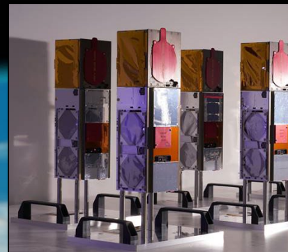
Constellation of Four 3U CubeSats MIT LL payload; BCT bus; KSAT downlink
