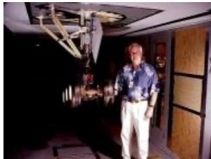
777 Landing Gear 1st large-scale gear noise data in U.S.
