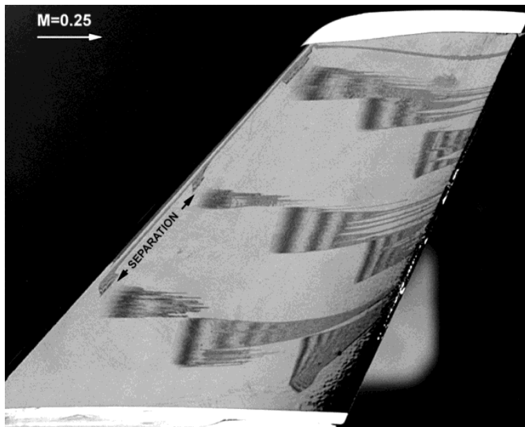
False-colored FISF image of a wing tip model showing the skin friction coefficient distribution at Reynolds number = 4.5 million and angle-of-attack = 10^\circ .
