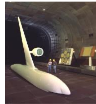
26%-Scale B-777 Large-scale application of microphone arrays in a wind tunnel
