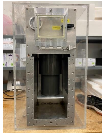
Figure 5. Front view of the Mpactor with front panel removed showing compaction chamber
