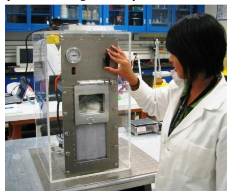
Figure 1. CEV Compactor (Now called the Mpactor)
