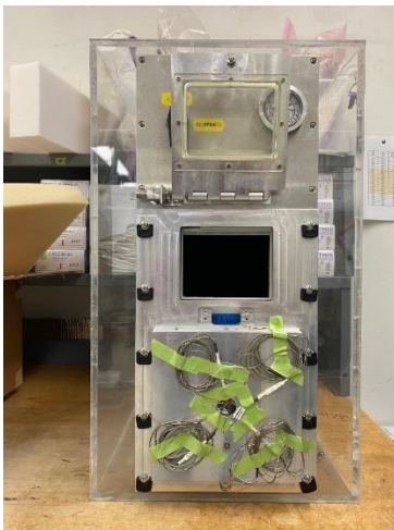
Figure 6. Front view of the Mpactor with front panel removed showing compaction chamber
