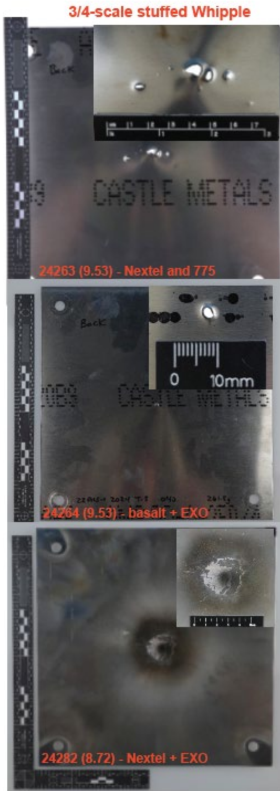
Figure 6. Post-test photographs of the backside of the witness plates from the three variants of the \frac{3}{4} -scale stuffed Whipple shield (label in bottom left, projectile size in parenthesis). Oblique views of damage provided as insets.
