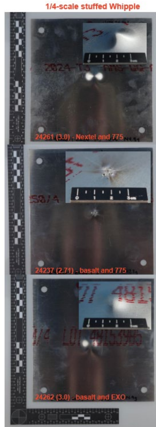
Figure 5. Post-test photographs of the backside of the rearwall from the three variants of the 1/4-scale stuffed Whipple shield (label in bottom left, projectile size in parenthesis). Oblique views of damage provided as insets.
