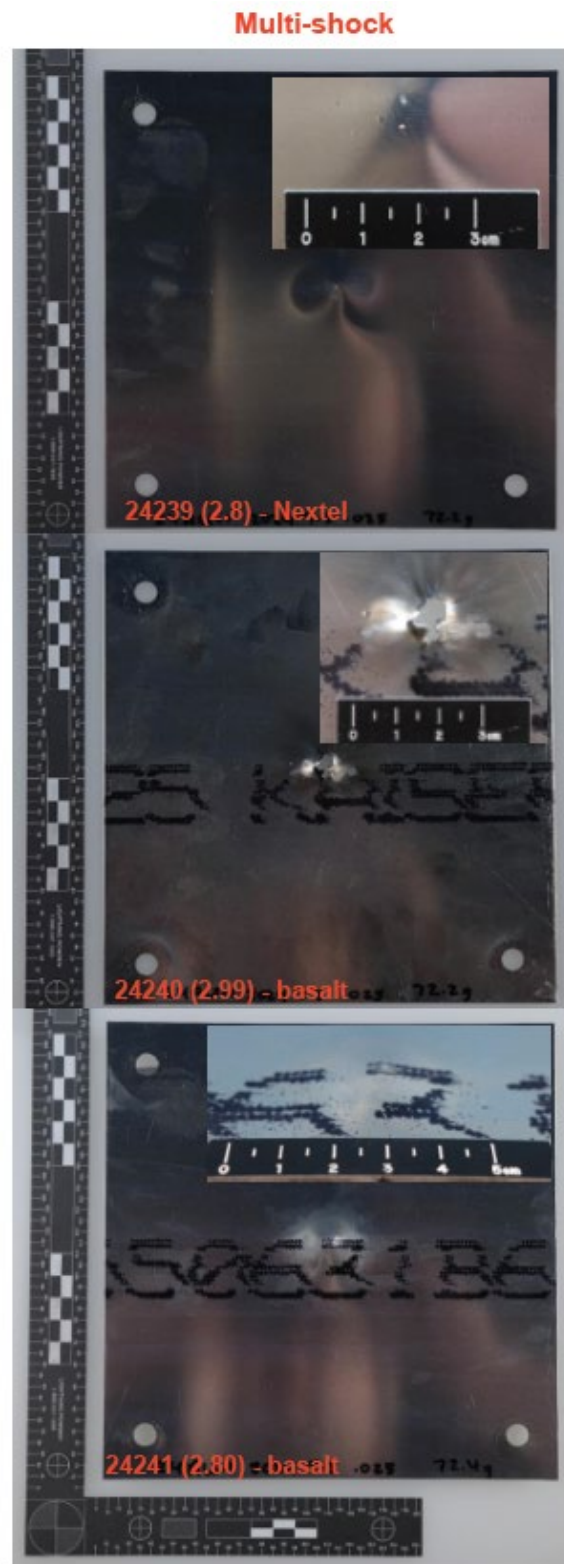
Figure 4. Post-test photographs of the backside of the rearwall from the three variants of the multi-shock shield (label in bottom left, projectile size in parenthesis). Oblique views of damage provided as insets.
