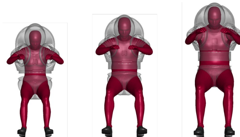
Figure 2: 5 th female, 50 th male, and 95 th male percentile GHBMC models posed into a seated configuration.
