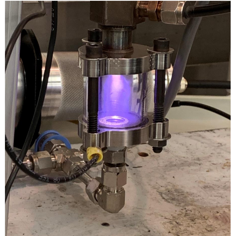
DC, nitrogen plasma torch in a quartz cell.
