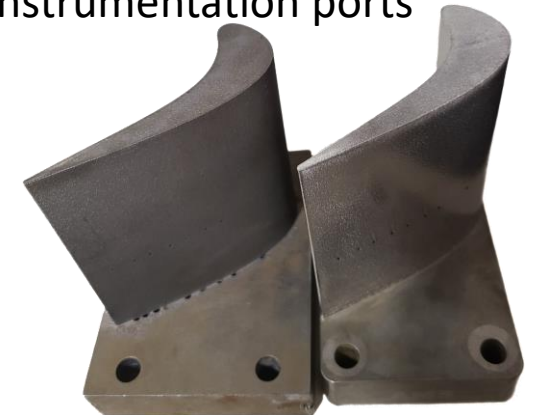
Turbine Blade with integral instrumentation ports
