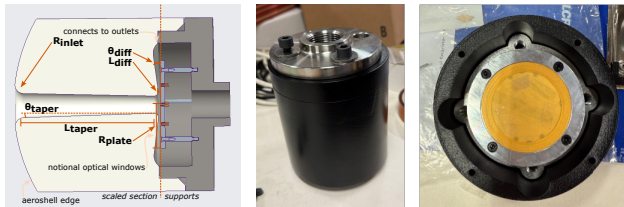
Figure 3. (l) Cutaway schematic of the test article; (c) small-scale test article, inlet facing down; (r) back portion of test article (inlet removed) exposing the collector assembly.
