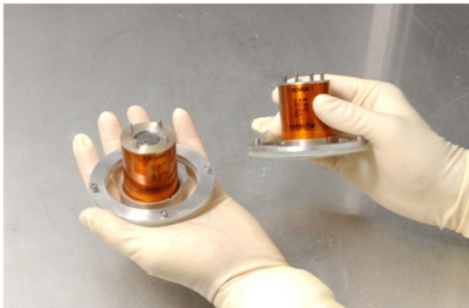
Passive Thermal Control Heat Switch. Shown here are heat switches with dust cover shields.
