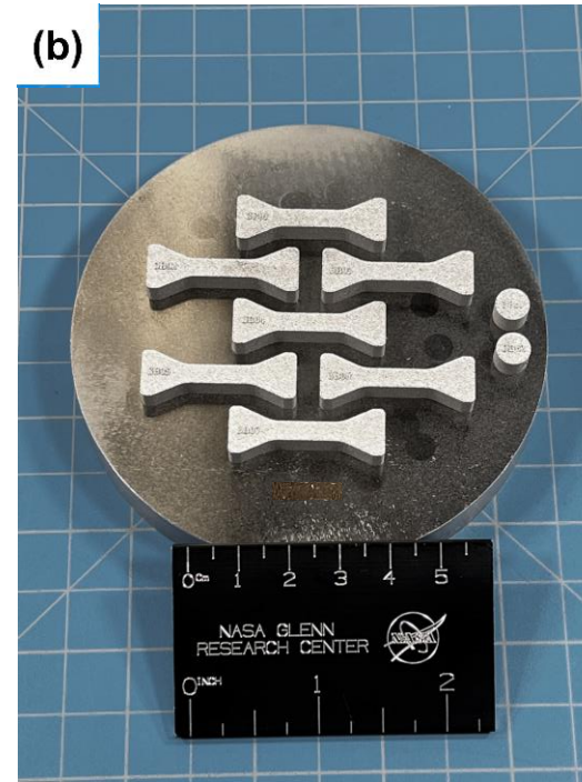
(a) Schematic L-PBF build layout and (b) image of the completed C103 build
