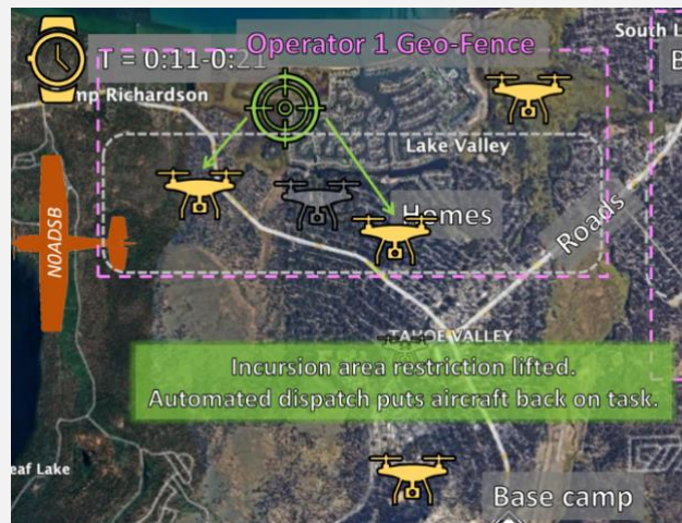
Figure 6: Following an aircraft incursion, restrictions are lifted and aircraft are automatically re-dispatched back to their tasks, illustrating the seamless integration of exception management with operational continuity.
