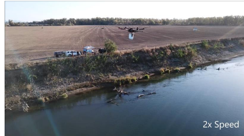
A UAV maps the flow field of the Sacramento River using RiOS
