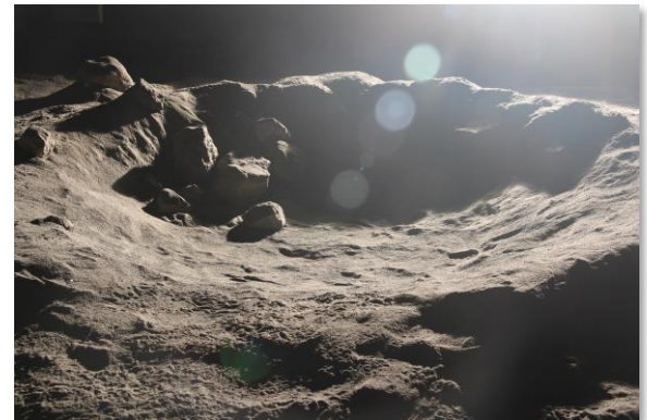
Physical simulation of crater features and high dynamic range solar illumination
