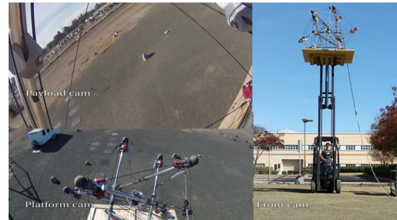
Video: SUPERball dropping from a tall platform and rolling away.
