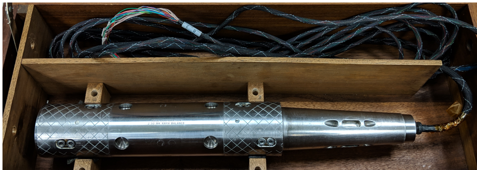
Fig. 8-1 NASA's 2.5 inch diameter MK34 six-component force balance.
