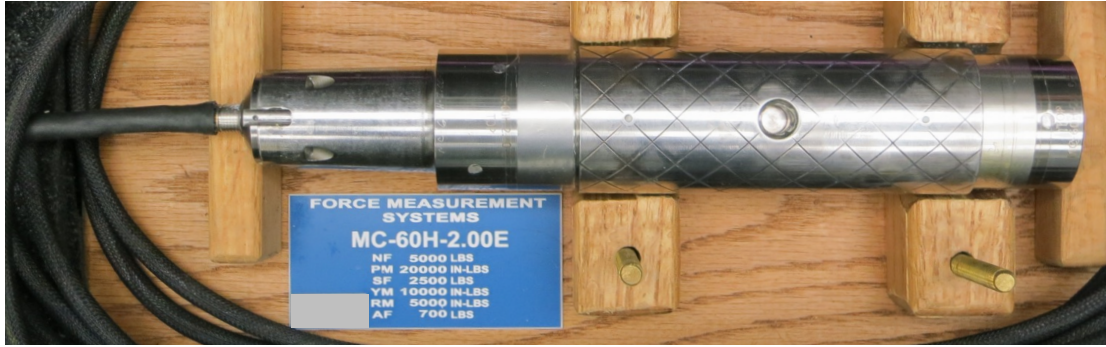
Fig. 7–13 NASA’s 2.0 inch diameter MC60E six–component force balance.
