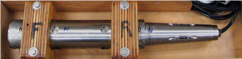
Fig. 33 Basic layout of NASA’s 2.5 inch MK40A force balance.
