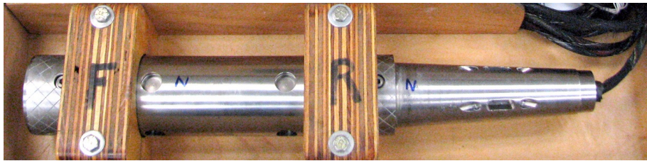
Fig. 24–2 NASA’s MK40A six-component force balance.
