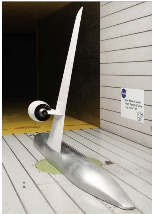
Fig. 55 Installation of the UHB semi-span model in the Ames 11-ft TWT.
