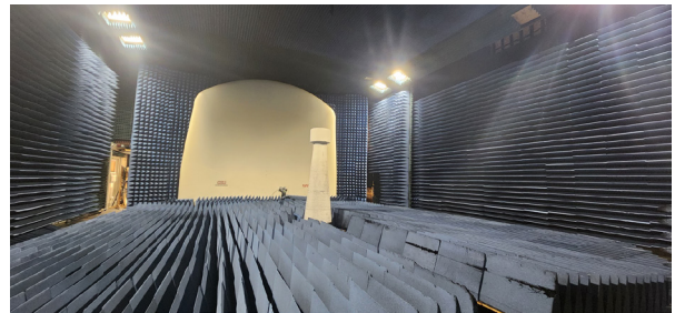
Figure 2. OSU-ESL radar range with the rotating foam test positioner in the center of the image.
