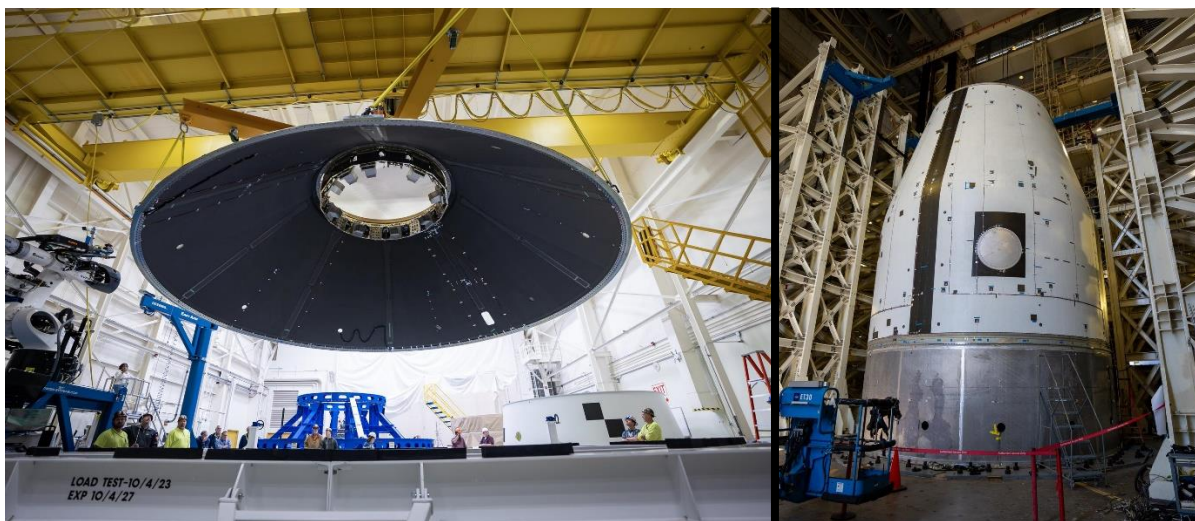
Fig. 5 The payload adapter (left) and universal stage adapter (right) will be able to house large co-manifested payloads as well as CubeSat secondary payloads on the Block 1B and Block 2 variants. Note the Nest ring inside the top opening of the payload adapter.
