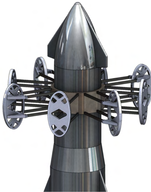
Figure 2.1: Rendering of the CREW HaT active magnetic shielding concept attached to SpaceX Starship’s crew habitat.
