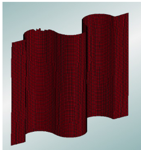
Figure B.23.—Typical crushing failure pattern at 13 mm of crush for sinusoid specimen.
