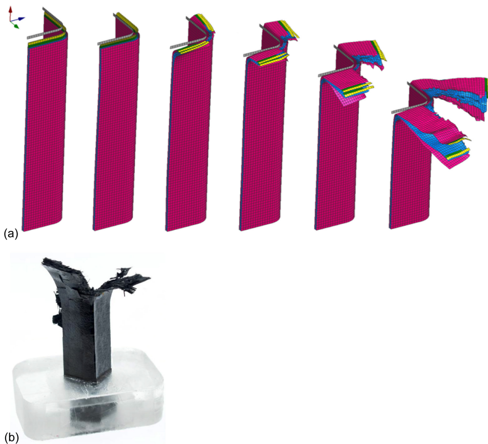
Figure B.30.—Small angle specimen crushing response. (a) Numerical model crushing process sequence. (b) Experimental result.
