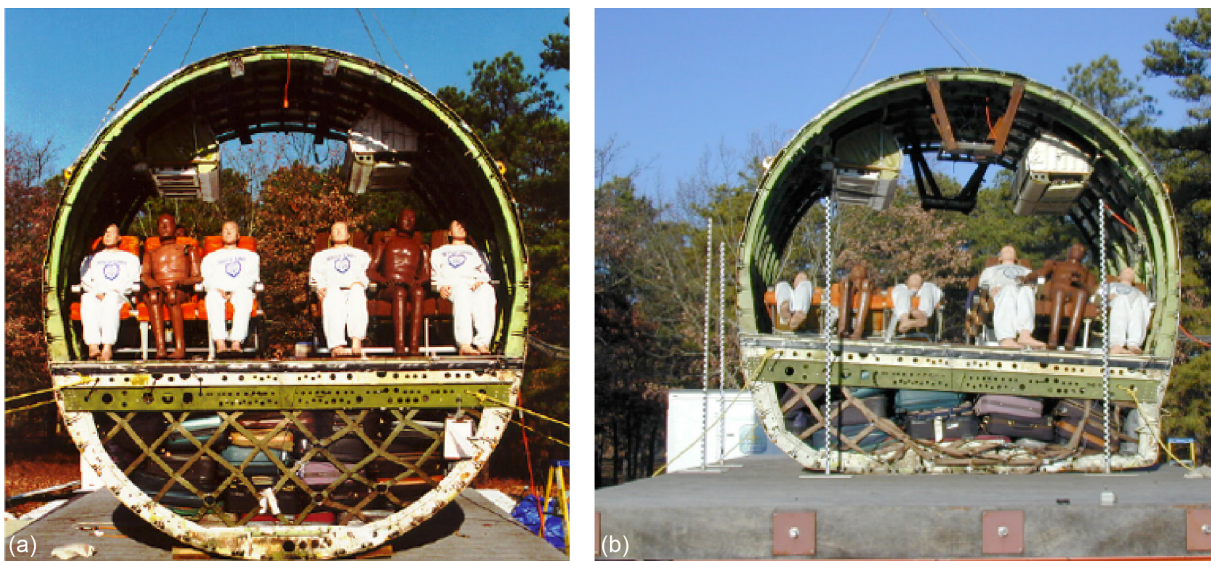
Figure 5.—Drop test of 737 fuselage section with underfloor luggage. (a) Test configuration. (b) After impact.
