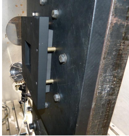
Figure 123.—Test specimen support fixture for measuring dent depth and extent of impact damage.
