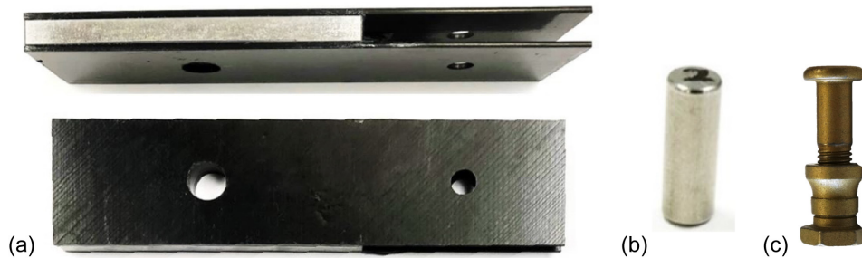
Figure 132.—Test article assembly for joint testing. (a) CRFP laminates and spacer. (b) Titanium pin. (c) Bolted fastener.
