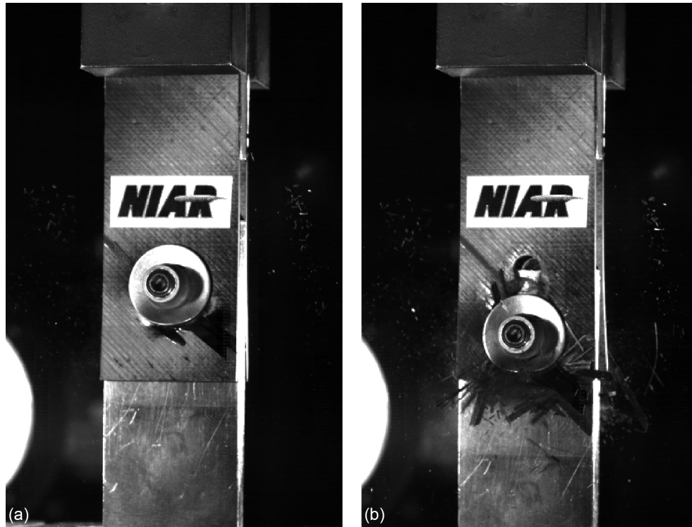
Figure 137.—Results of bolted fastener joint testing conducted at 100 in./s. (a) Surface ply splitting. (b) Bending of washers due to debris accumulation and failed composite fragments.
