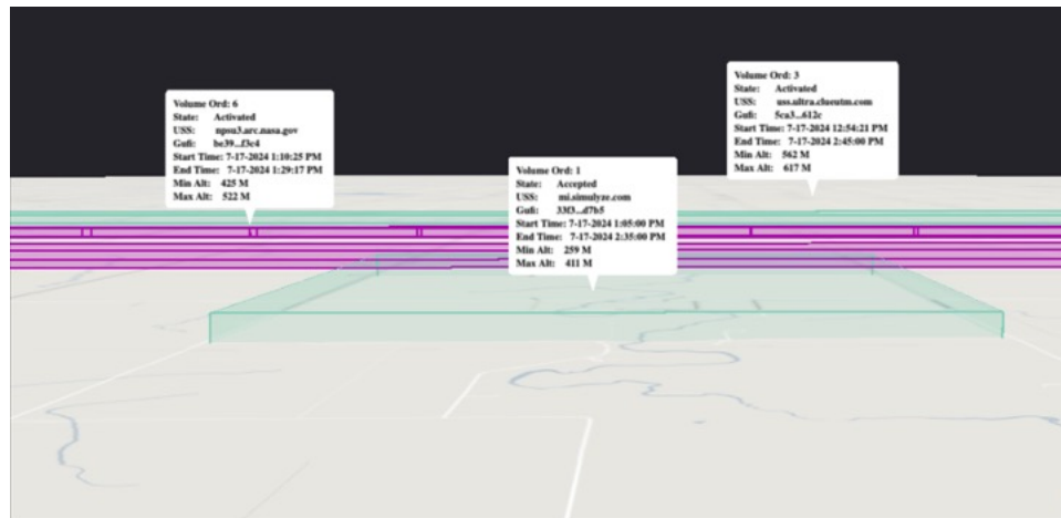
Figure 8. Side-view of XTM1 and CLUE1's active (magenta) volumes with 40m vertical separation.
