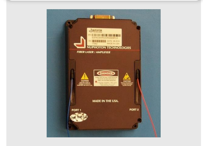
~1 W Erbium Doped Fiber Amplifier Optical C-Band (~1550 nm)
