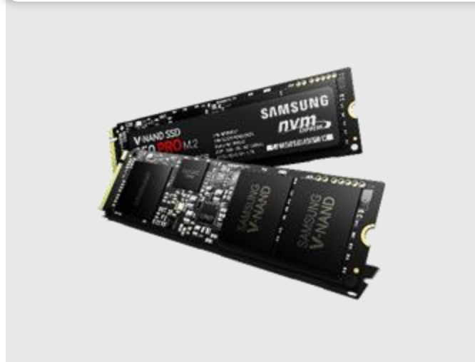
>500 GB, >25 Gbps Readout Solid-State Drive (SSD)
