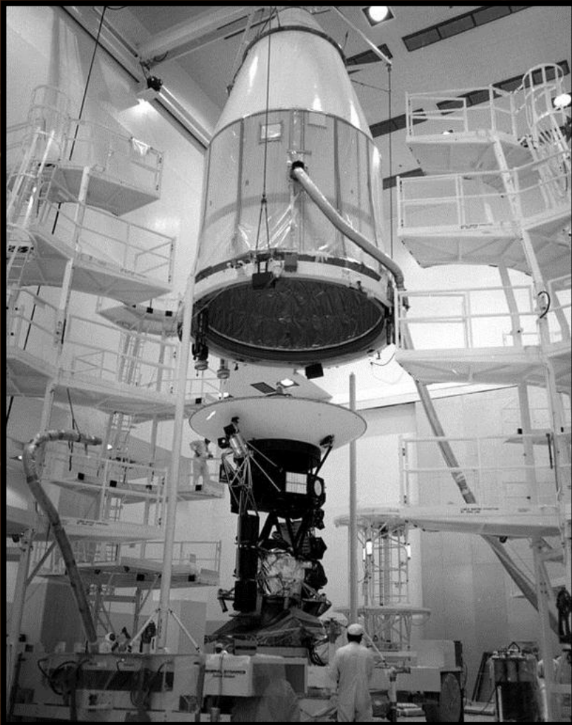
3.7-m antenna— largest antenna that can fit in rocket fairing
