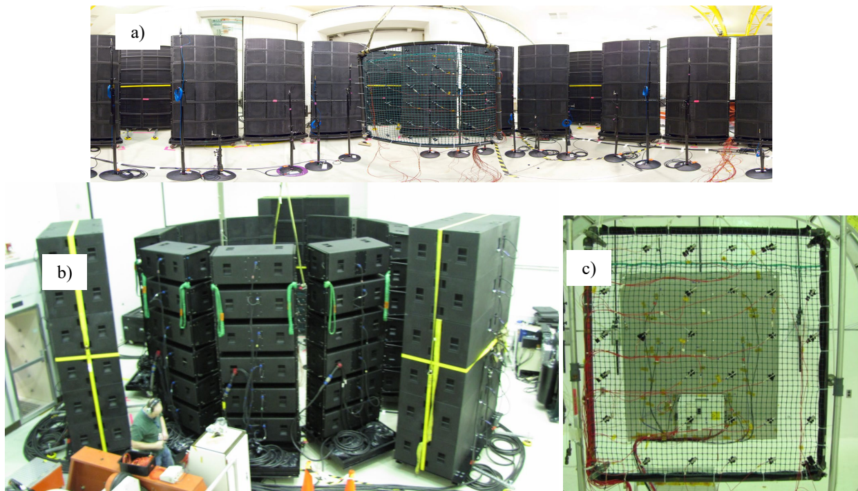
Figure 1: (a) Speaker and woofer arrangement captured with a wide-angle camera, (b) speaker testing volume used in JPL tests, and (c) microphone array setup.
