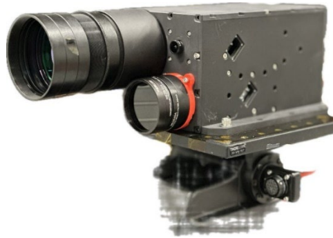
Figure 6. Terrain Sensing Lidar (TSL) prototype with multi-functional capability.
