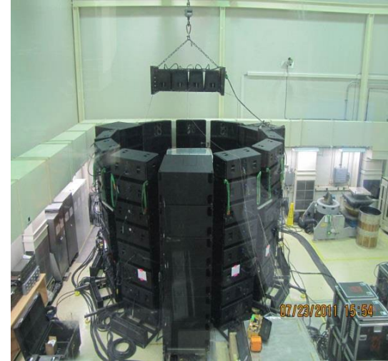
(a) APL speaker and woofer arrangement with control microphones, microphone array, and linear array. (b) Photograph of the APL DFA test setup
