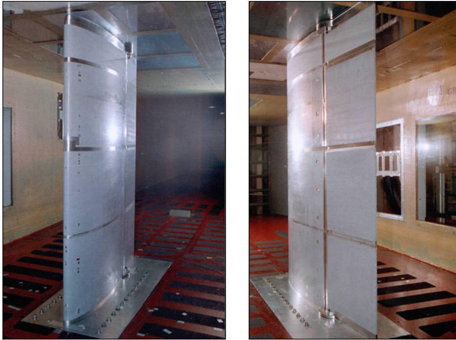
Figure 1.1: Twin Otter Airfoil Model Installed in the IRT
