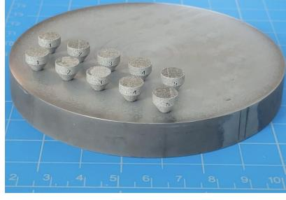
Example of parameter optimization sample burnout at build plate interface
