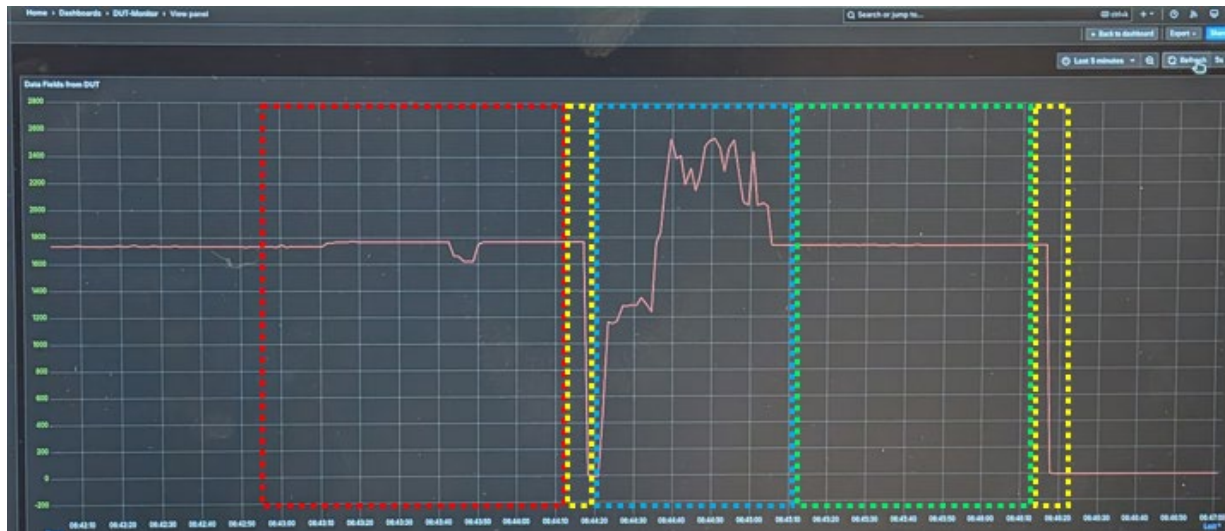
Figure 5: Exemplar Grafana Dashboard showing Current Draw at Different Modes of Operation (Red – Single Event Functional Interrupt, Yellow 1 - Power Cycle, Blue- Boot Process, Green - Idle Operation, Yellow 2 – Power Off)
