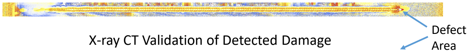
In-situ NDE Inspection Image using Principal Component Analysis
