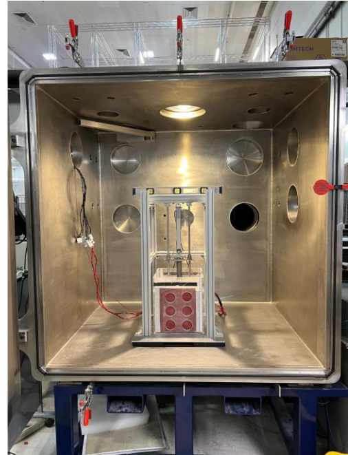
Figure 1. Pressure Sinkage Test Rig in a NASA Vacuum Chamber
