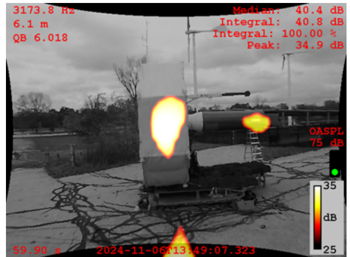
FIGURE 18: OVERALL SOUND PRESSURE LEVEL FIELD FOR A FAN SPEED OF 800 RPM, AN ADVANCE RATIO J = 0.19 , AND WIND ALIGNMENT \theta_{align.} = -5^\circ .
