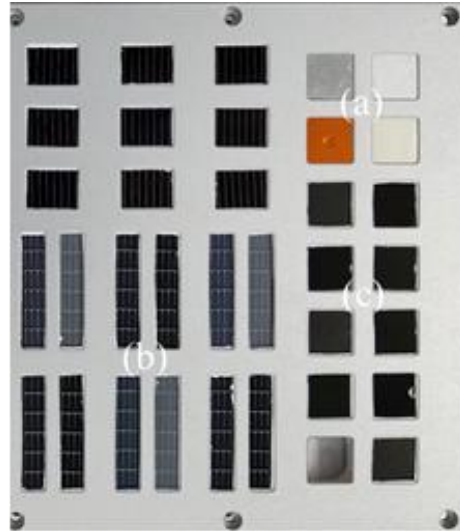
Figure 2: LISA-T MISSE-FF mission plate (a) bare materials and witness samples, (b) copper indium gallium (di)selenide solar cells, (c) inverted metamorphic multijunction solar cells.
