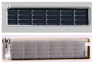
Figure 10: Enlarged view of Pre- (a) and Post-flight (b) images of CORIN XLS with glass additive coated CIGS modules.
