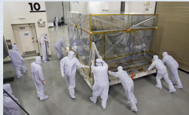
The InSight spacecraft has been removed from its shipping container and is being moved for removal of protective wrapping.
